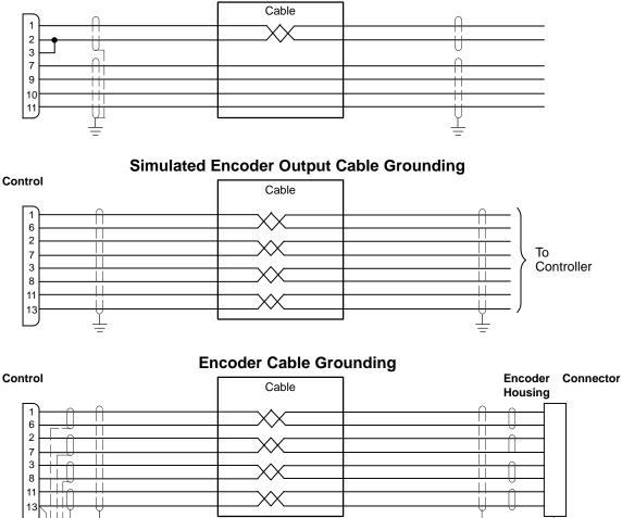
Input Signal Cable Grounding
